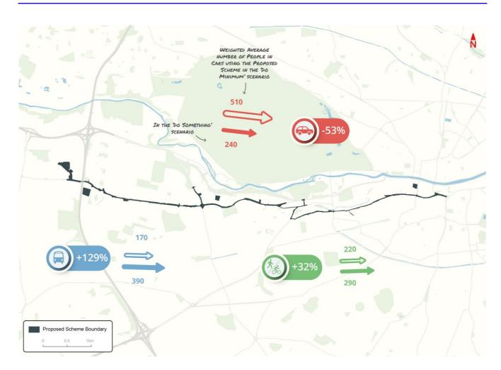
Diagram 6.9: People Movement by Mode travelling along the Proposed Scheme during 2043 AM Peak Hour
