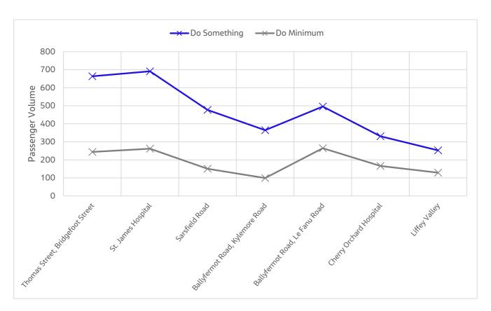
Diagram 6.14: 2043 PM Peak Hour Passenger Volume Along Proposed Scheme (Outbound Direction)
