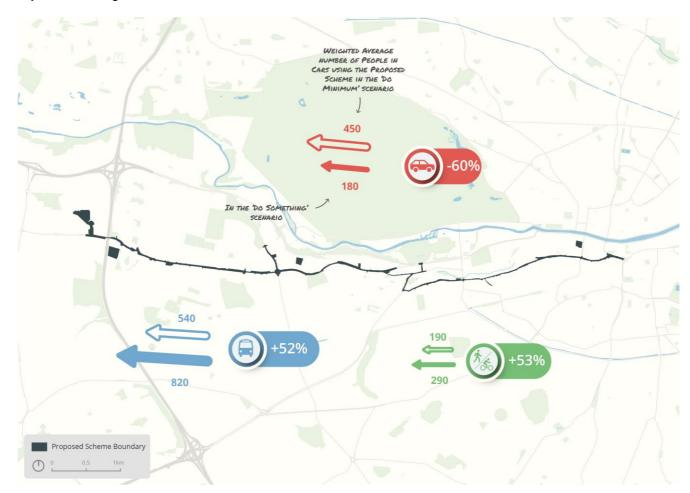
Diagram 6.8: People Movement by Mode travelling along the Proposed Scheme during 2028 PM Peak Hour
