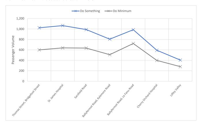
Diagram 6.12: 2028 PM Peak Hour Passenger Volume Along Proposed Scheme (outbound direction)
