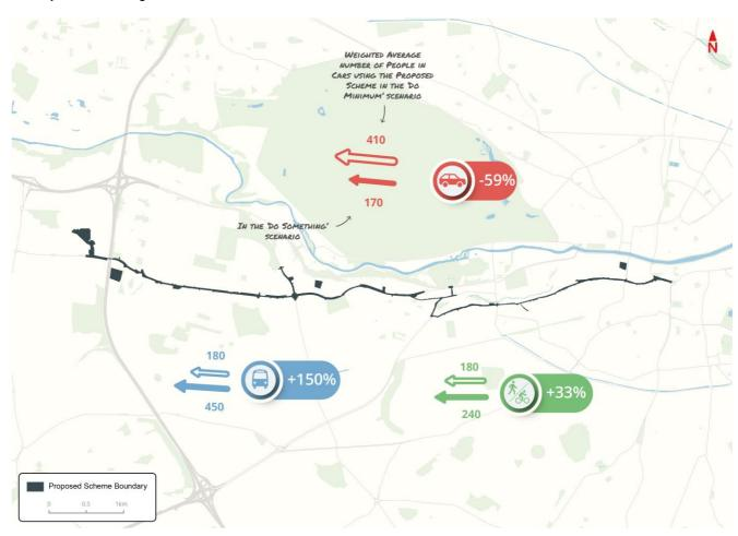
Diagram 6.10: People Movement by Mode travelling along the Proposed Scheme during 2043 PM Peak Hour
