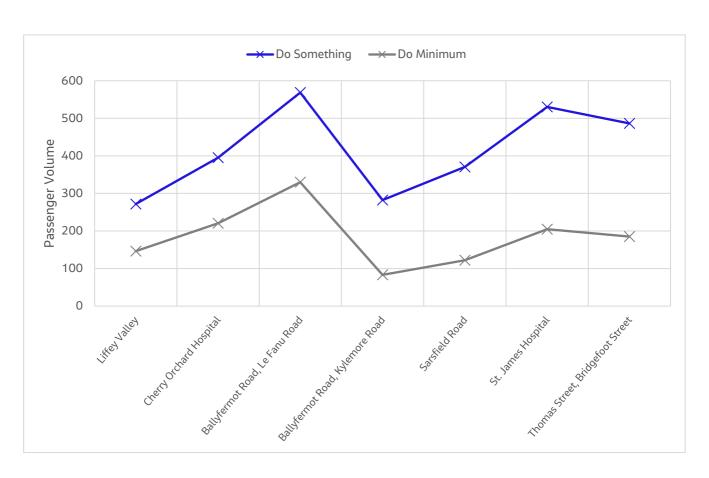
Diagram 6.13: 2043 AM Peak Hour Passenger Volume Along Proposed Scheme (outbound direction)
