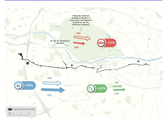
Diagram 6.7: People Movement by Mode travelling along the Proposed Scheme during 2028 AM Peak Hour
